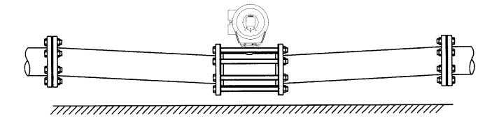
Figure 4.3 Model Diagram of Unsupported Pipes
